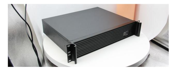
The 8F2E1 artificial intelligence computing platform (hereinafter referred to as 8F2E1) is equipped with NVIDIA Jetson AGX Orin/AGX Xavier core modules. It can provide up to 275 TOPS of computing power, which can be widely used in education, industrial automation, smart city and other scenarios. With a wealth of external interface, internal interface devices are wide temperature model.
